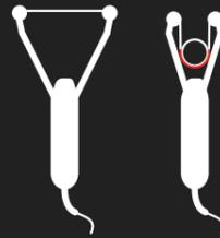
Suitable for easy, efficient and even grinding and polishing of round surfaces such as handrails, drainpipes, furniture parts. The spring-loaded arm adjusts as the belt is pressed against the workpiece, the force required is adjustable. Variable speed. With anti-vibration handle, overload- and restart protection. Lock-on switch.
